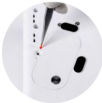
② Pry out the base cover from the slot with tweezers
